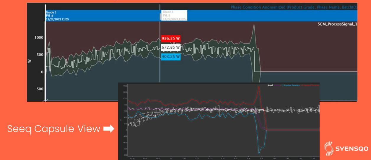
Define the ideal profile of a process variable throughout a batch as well as an acceptable/reference envelope based on statistics
