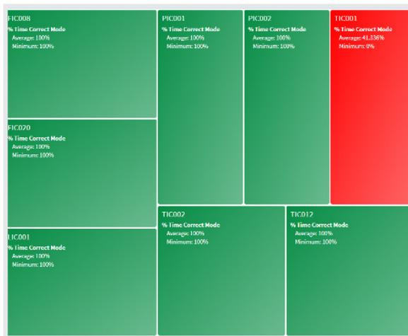
This image shows a treemap that includes several controllers. The treemap is colored based upon which controllers are running in their correct mode. This is a helpful tool in giving a quick, high-level overview of how the assets (controllers) are performing.
