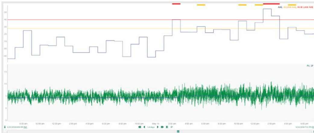
The bottom lane shows a controller’s process variable and setpoint. Looking at the trend, it may not be immediately obvious that anything has changed in the controller’s performance; however, the top trend shows the calculated Average Absolute Error (AAE) of the controller, which is clearly increasing over time. This increase in AAE may be due to a change in operating level.
