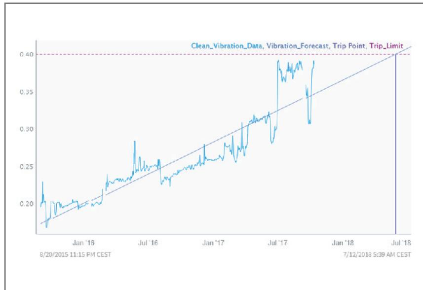
The figure shows a Seeq Analysis with a vibration signal on an induced-draft fan and a predicted vibration forecast.
